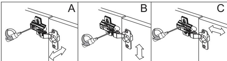
A. Lateral adjustment by screw adjusting    B. Vertical adjustment via slot in the mounting plate    C. Front-to-Back by the slacking the hinge arm mounting screw
