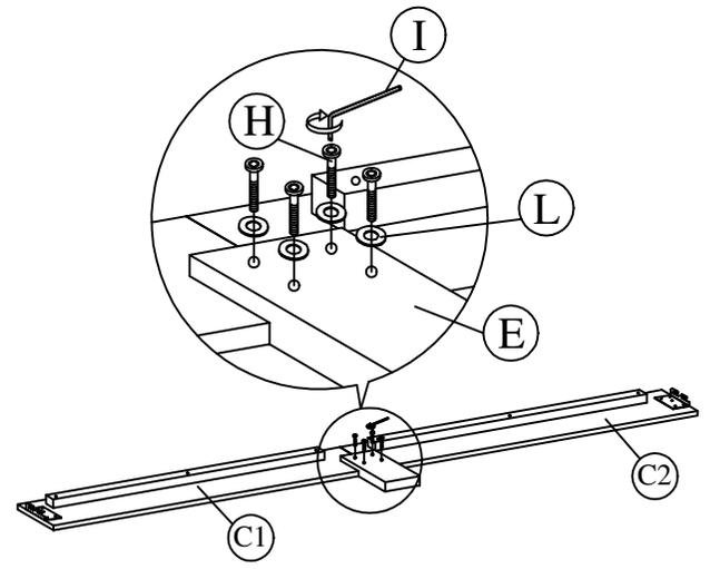
Step 4 : Attach side rail (C) to headboard (A) and footboard (B) by pushing the bracket down to fit it.
