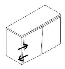
**Lateral Adjustment** by adjusting screw
